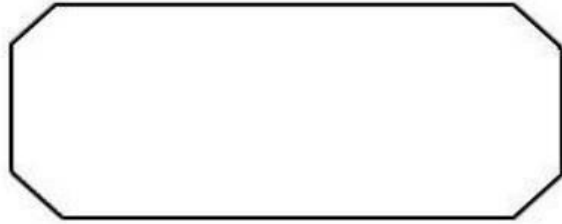
Loop Area corner Cut 45 Degree (Recommended)
