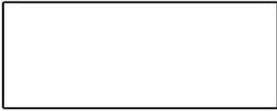
Loop Area corners Cut 90 Degree (Not Recommended)
